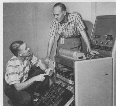
**VERSATILE OPERATION of the "Blue Boy" Automatic Program**mer and Recorder is made possible by these trays of interchangeable transistorized cards. Circuit arrangement of one of the cards is discussed by Robert Adams (L) and Clinton Purdue (both 1521).
